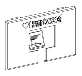
3. Press down on the top of the cat jack and twist the top into place.
