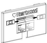
Hook the top raceway grommet tabs onto the raceway edge, push raceway grommet up and in to position on the raceway cover.
