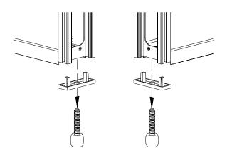
3. Remove all male connecting hooks from the connecting side pillar of one of the two panels.
