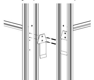
4. Line up the female connecting hooks with holes indicated below. Install one female connecting hook in each instance where a male connection hook was removed. Secure the female connecting hooks with screws removed in Step 3.
