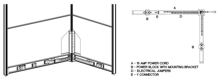
Example A - shows a ceiling power feed cable and a jumper cable connecting on the same side of a power block.
