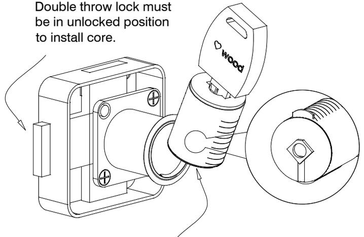
Install with key inserted in core. Align the two diamond shapes on both the bottom of the core and inside the lock housing. Tilt core at an angle and slide into housing until core **snaps** in place.
