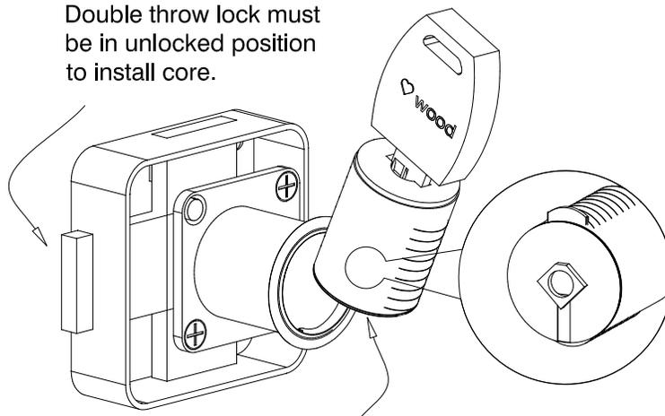
\*The core can be removed with the red removal key. The lock must be in the unlocked position to remove the core.
