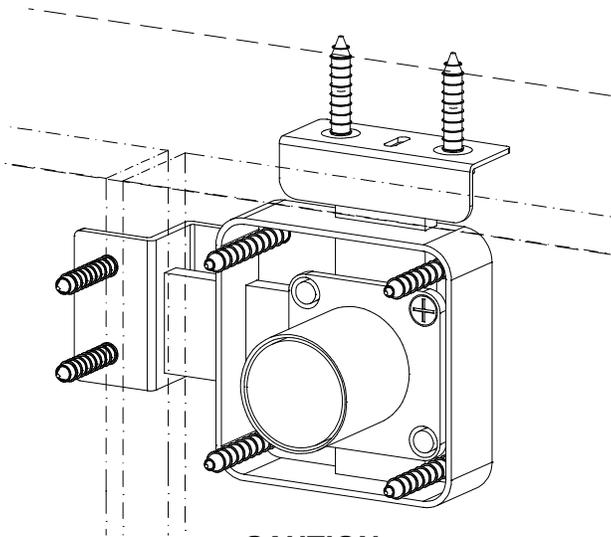
Double throw lock must be in unlocked position to install core.
