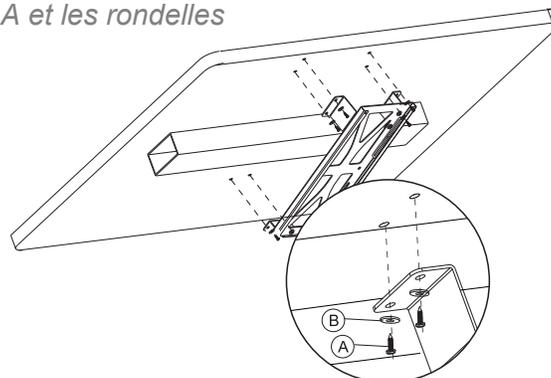
**STEP 1 - Option C: Install panel to worksurface using the corner connectors /**
