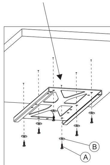
**STEP 1 - Option B: Install panel to worksurface using the corner connectors /**
